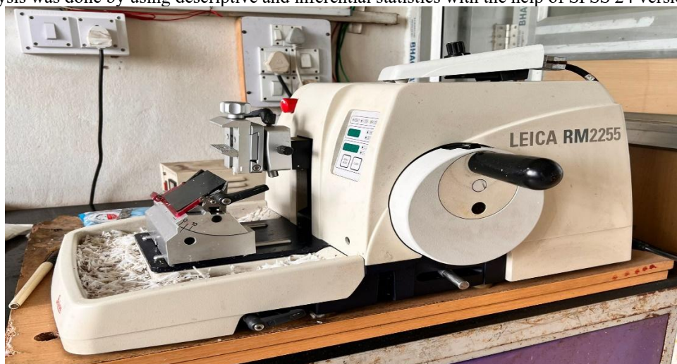
Figure 1: Rotatory microtome (Leica rm2255) use for sectioning of paraffin embedded specimens
